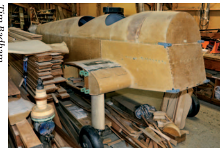
The wooden construction is evident in this example being restored in New Zealand
