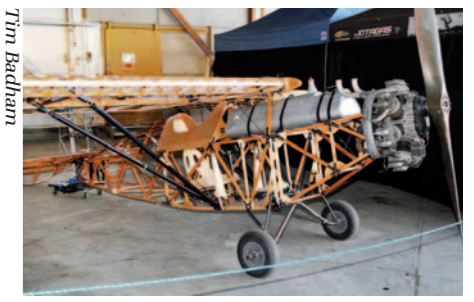
The structure includes a surprising amount of complex metalwork. This is Swift VH-UVC when being restored in New Zealand.
